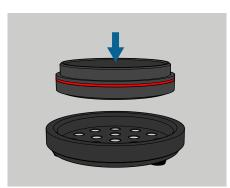
Put the red marked (smaller) part of the adapter with the marking line downward on the saturation plate, covered with a filter paper.
