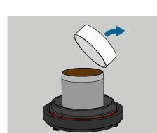
Turn the soil sample and remove the other lid. Place the soil sample in a water pan.
