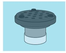
When the saturation is completed, close the soil sample with a lid, turn the whole system upside down and put it in a pan. (If there is only one soil sample in the saturation pan you can leave it there)
