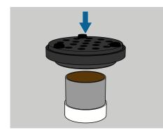
Flip the adapter and place it on top of the soil sampling ring.
