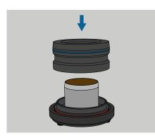
Put the blue marked (bigger) part of the adapter air free with the marking line upwards on top of the soil sampling ring.
