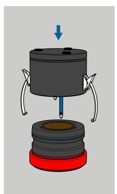
Put the refilled HYPROP<sup>®</sup> (for instructions about the preparation of the HYPROP<sup>®</sup> please read the HYPROP<sup>®</sup> manual) on top of the soil sample, turn the system upside down, remove the saturation plate and close the HYPROP<sup>®</sup> clips. Cover the soil sample with a lid to prevent evaporation before start of measurement.
