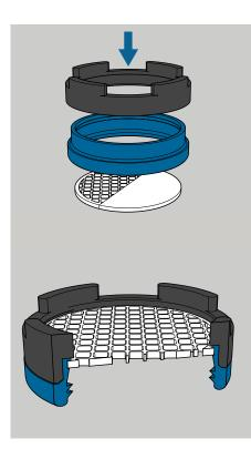
Press the porous plate or the mesh into the groove from the bottom of the blue gasket.
