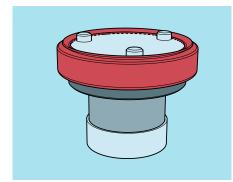
Saturate the porous plate of the red sealing (see note on next site) and put it in the same water filled pan.
