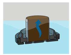
Fill the pan with water until it is just below the top of the sample ring (recommended times see below). Carefully tilt the sample including the saturation plate to let escape air bubbles.
