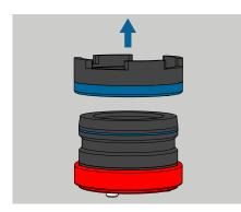
For continuing with a HYPROP<sup>®</sup> measurement open the burette cock and remove the system from the KSAT.
