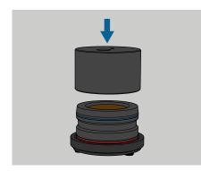
When the saturation is done take the soil sample out of the water pan and put the auger guide on top of the blue marked part of the adapter for augering the holes for the tensiometer shafts.
