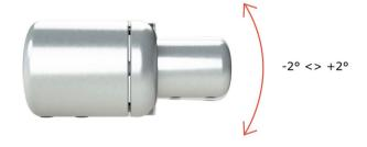
**Figure 2** ALF01 albedometer levelling tool, can be rotated around the axis of the crossarm to which it is connected, and tilted over  $\pm$  2 °.
