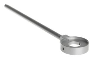
**Figure 1** AMF02 or AMF03 albedometer kits are used to mount both an up- and a downfacing pyranometer, and construct an albedometer. The image shows the AMF02 mounting fixture and its rod. A glare screen for the downfacing sensor is also included.
