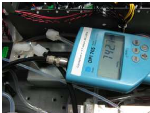
Figure 79 – Disconnect inlet of Photometer
