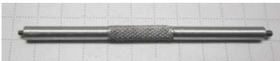
Figure 85 – Orifice Removal Tool – H010046
