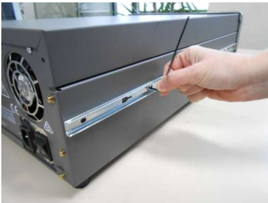
Figure 98 – Assemble Inner Slide on Chassis
