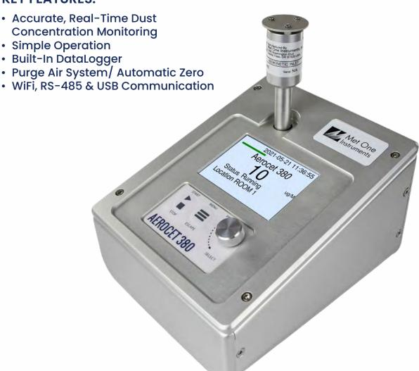
The Met One Instruments, Inc Aerocet 380 is a nephelometer that offers real-time airborne TSP (total suspended particulate) concentration levels using the principle of forward laser light scatter. This instrument is ideal for sampling in any indoor workplace or public place environment with optional separators to monitor PM<sub>1</sub>, PM<sub>2.5</sub>, or PM<sub>10</sub>.
