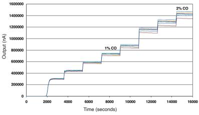
Figure 3 shows the excellent response to step changes in CO concentrations from zero to 2% CO by volume.
