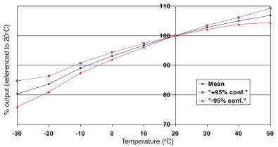
Figure 1 shows the variation in sensitivity caused by changes in temperature.
