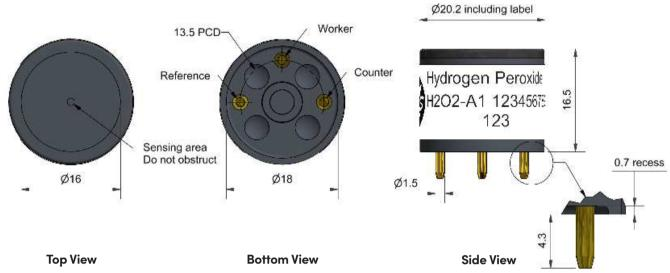
Dimensions are in millimetres (± 0.1 mm).
