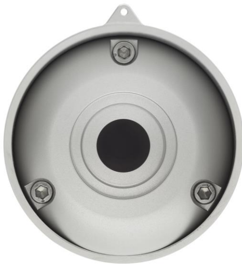
Figure 1.3.1 DR30 first class pyrhelimeter front view; window assembly with heater
