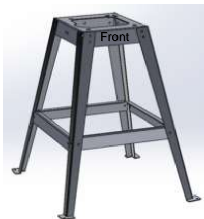
Figure 3-3 E-FRM-DC Sampler Stand Final Assembly
