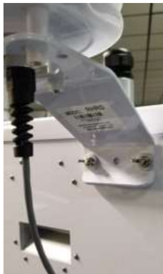
Figure 3-5 Ambient Temperature Sensor Assembly Mounting
