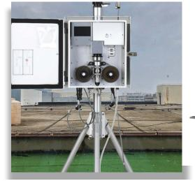
The Met One Instruments, Inc. E-BAM Plus is a portable, real-time beta gauge is a U.S.-EPA designated equivalent method for  $PM_{10}$ .
