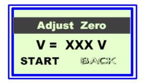
In this case adjust by the Zero Potentiometer on the back the Voltage to V < 0,10V
