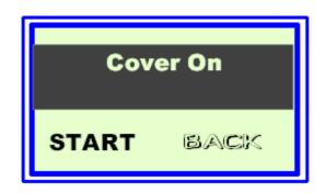
In the dark field it shows an advice to set the cover (protection cap) onto the modulator system. Press the " $\leftarrow \rightarrow$ " Button (4) to select **START** or **BACK**.
