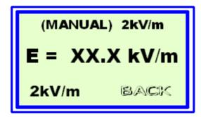
In the 1st. line it shows the selected Measure Mode => **MANUAL** and the Selected Range => **2kV/m**.
