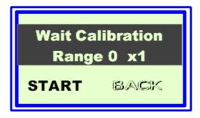
The buttons are out of function during the Zero procedure.
