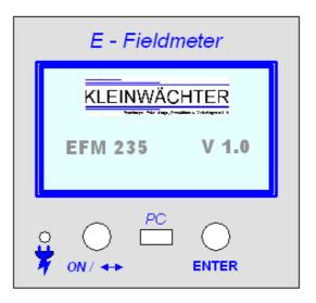
It shows the Type = EFM 235/EFM 255 and the Version Number V X.X After that, the unit switches to:
