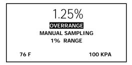
Once the OVER RANGE warning appears the user must advance the transmitter to the next higher range. **NOTE:** With oxygen reading above 110% of the selected range, the analog signal output will increase but will freeze at a maximum value of 1.2 V. After the oxygen reading falls below the full scale range, the voltage signal will become normal.
