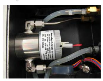
Unscrew the old sensor and screw in the new sensor finger tight
