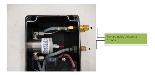
As illustrated above, the GPR-1000's internal sample system includes:
