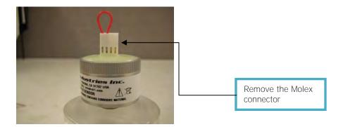
Connect the sensor with the sensor cable and hold the sensor in your hand for a couple of minutes to allow the sensor to stabilize with ambient air.
