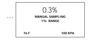
If the oxygen value goes above the 1%, display will not shift to the next higher range. Instead, when the oxygen reading exceeds 110% of the upper limit of the current range, an OVER RANGE warning will be displayed.
