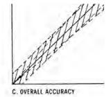
**Example:** As illustrated by Graph A, any error due to the tolerances in the circuit, will increase with increasing oxygen concentration if the analyzer calibration is done at lower end of the range, e.g., calibration with 20.9%, any error would be multiplied by a factor of 4.78 (100/20.9) when used for measurements near 100% oxygen. Conversely, an error during a span adjustment at 100% of full scale range is reduced proportionately for measurements of lower oxygen concentrations.
