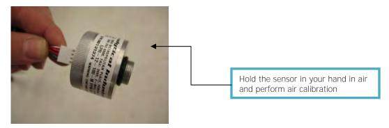
After air calibration, screw the sensor in the sensor housing and immediately allow the sample or zero gas to flow through the sensor housing.
