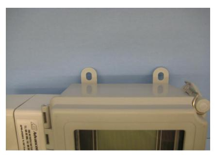
The transmitters design provides protection from RFI that is maintained by leaving specific mating areas of the enclosure unpainted to maintain conductivity of the gasket, top and bottom sections of the smaller enclosure housing the electronics. These unpainted areas are protected by gaskets and contribute to maintaining the NEMA 4 rating as well as protection from RFI/EMI. Do not paint these areas.
