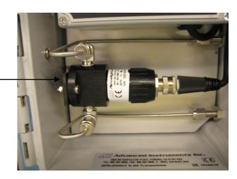
Delrin Senor Housing with sensor installed.
