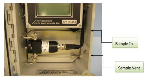
Flow rates of 1-5 SCFH cause no appreciable change in the oxygen reading. However, flow rates above 5 SCFH generate backpressure and erroneous oxygen readings because the diameter of the integral tubing cannot evacuate the sample gas at the higher flow rate. A flow indicator with an integral metering valve upstream of the sensor is recommended as a means of controlling the flow rate of the sample gas. A flow rate of 1-2 SCFH or 0.4-1 liter per minute is recommended for optimum performance.
