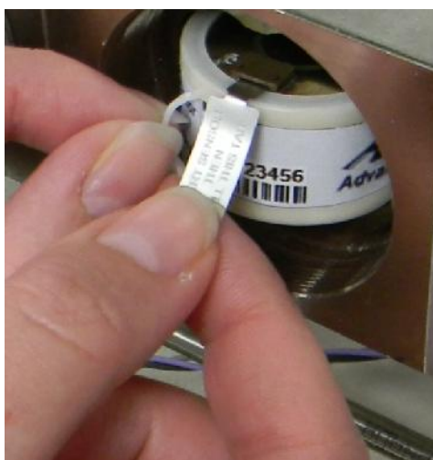
Figure 9. Inserting sensor in cell block
