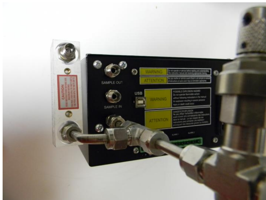
Figure 8 Span gas bypass connection – back view.
