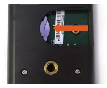
The positive side (designated by a "+" sign) should be facing out from the meter circuit board.
