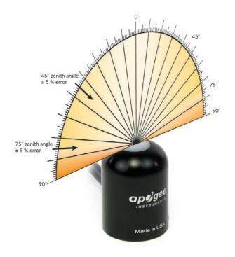
Directional, or cosine, response is defined as the measurement error at a specific angle of radiation incidence. Error for Apogee silicon-cell pyranometers is approximately  $\pm$  2 % and  $\pm$  5 % at solar zenith angles of 45° and 75°, respectively.
