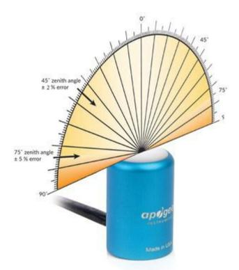
Directional (cosine) response is defined as the measurement error at a specific angle of radiation incidence. Error for Apogee MQ-500 series quantum sensors is approximately  $\pm 2$  % and  $\pm 5$  % at solar zenith angles of 45° and 75°, respectively.
