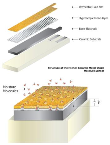
**Operation of the Michell Ceramic Metal-Oxide Moisture Sensor**
