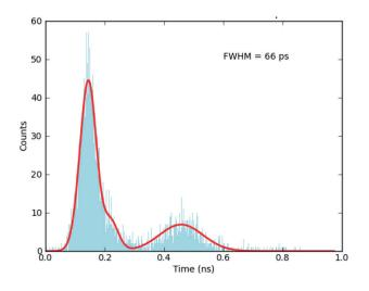
\*Results taken from J. Milnes et al., Recent Developments in Ultra-High Speed and Large Area Photomultiplier Tubes, PoS(ECPD2015)005 of a 1 MCP, 10 mm PMT.
