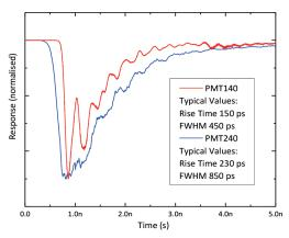
The figure below shows the influence of the laser pulse width and measurement bandwidth on the observed result.\*
