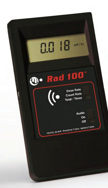
The Rad 100<sup>™</sup> measures Alpha, Beta, Gamma, and X-radiation. Its digital display shows readings in your choice of counts per minute (CPM), µSv/hr or mR/hr, or in accumulated counts. A red LED blinks and a beeper chirps with each count (the chirp can be muted).
