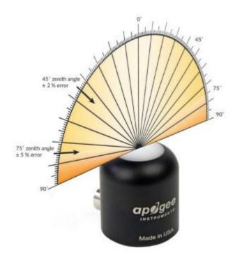
Directional (cosine) response is defined as the measurement error at a specific angle of radiation incidence. Error for Apogee S2 series PAR-FAR sensors is approximately  $\pm$  2 % and  $\pm$  5 % at solar zenith angles of 45° and 75°, respectively.
