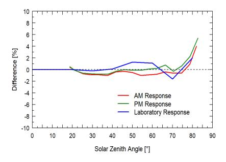
Mean directional (cosine) response of seven apogee PAR-FAR sensors. Directional response measurements were made on the rooftop of the Apogee building in Logan, Utah. Directional response was calculated as the relative difference of PAR-FAR sensors from the mean of replicate PAR detectors (LI-COR models LI-190 and LI-190R, Kipp & Zonen model PQS 1). Data were also collected in the laboratory using a reference lamp and positioning the sensor at varying angles.
