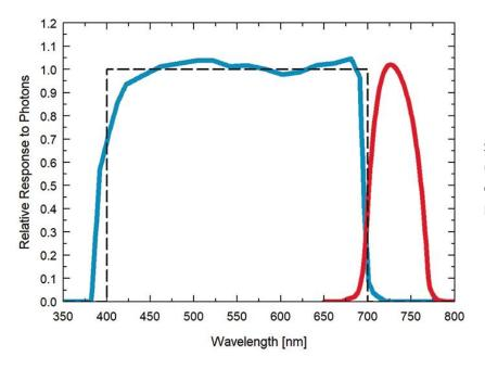
Spectral response of PAR detector (blue) and Far-red detector (red) compared to the defined response of plants to photons (dashed).
