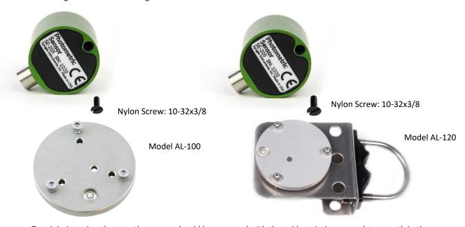
To minimize azimuth error, the sensor should be mounted with the cable pointing toward true north in the northern hemisphere or true south in the southern hemisphere. Azimuth error is typically less than 1 %, but it is easy to minimize by proper cable orientation.
