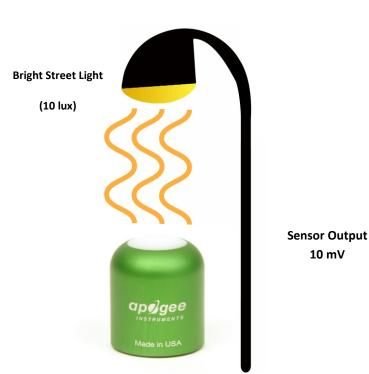
Example of illuminance measurement with an Apogee photometric sensor. Bright streetlights yield an illuminance on a horizontal plane at approximately 10 lux. This yields an output signal of 10 mV. The signal is converted to illuminance by multiplying by the calibration factor of 1 lux per mV.
