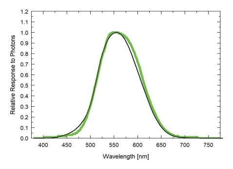
The mean relative spectral response of four SE-100 photometric radiometers (green) compared to CIE-1931 curve (dotted).
