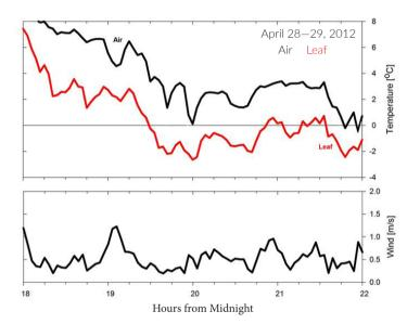
Leaf temperature approximations measured with an Apogee SF-110 compared to air temperature (top panel) and wind speed (bottom panel) on the evening of April 28, 2012. Leaf temperatures were below air temperature after 8 P.M. and reached freezing 6 hours before the air temperature.
