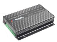
This datasheet covers four (4) product series (i.e. FA, FV, XA and XV series) of High-Precision Universal 2- and 4-Channel LED Controllers with External Triggers and 0.1mA Current Resolution, which currently include 8 models in total. All FA/FV/XA/XV LED controllers have 0.1mA current resolution, and a maximum current of 100mA in DC mode and 350mA in pulse mode.
