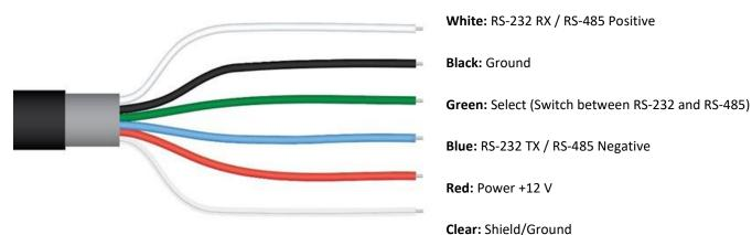
The green wire should be connected to Ground to enable RS-485 communication, or it should be connected to 12 V power for RS-232 communication. Text for the White and Blue wires above refers to the port that the wires
