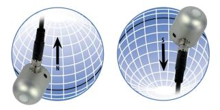
In addition to orienting the cable to point toward the nearest pole, the sensor should also be mounted such that obstructions (e.g., weather station tripod/tower or other instrumentation) do not shade the sensor. **Once mounted, the black cap should be removed from the sensor.** The green cap can be used as a protective covering for the sensor when it is not in use.
