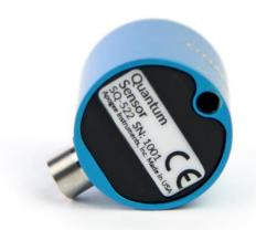
A sensor's model number and serial number are located on the bottom of the sensor. If you need the manufacturing date of your sensor, please contact Apogee Instruments with the serial number of your sensor.
