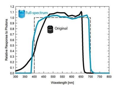
Mean spectral response measurements of six replicate Apogee SQ-100 (original) and SQ-500 (full-spectrum) series quantum sensors. Spectral response measurements were made at 10 nm increments across a wavelength range of 300 to 800 nm with a monochromator and an attached electric light source. Measured spectral data from each quantum sensor were normalized by the measured spectral response of the monochromator/electric light combination, which was measured with a spectroradiometer.
