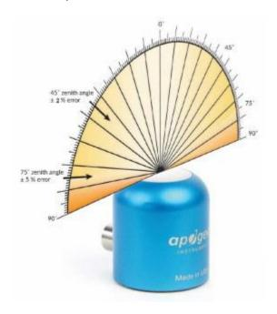
Directional (cosine) response is defined as the measurement error at a specific angle of radiation incidence. Error for Apogee SQ-500 series quantum sensors is approximately  $\pm$  2 % and  $\pm$  5 % at solar zenith angles of 45° and 75°, respectively.
