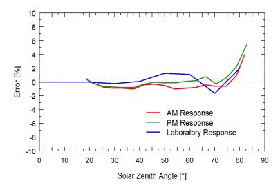
Mean directional (cosine) response of seven apogee SQ-500 series quantum sensors. Directional response measurements were made on the rooftop of the Apogee building in Logan, Utah. Directional response was calculated as the relative difference of SQ-500 quantum sensors from the mean of replicate reference quantum sensors (LI-COR models LI-190 and LI-190R, Kipp & Zonen model PQS 1). Data were also collected in the laboratory using a reference lamp and positioning the sensor at varying angles.
