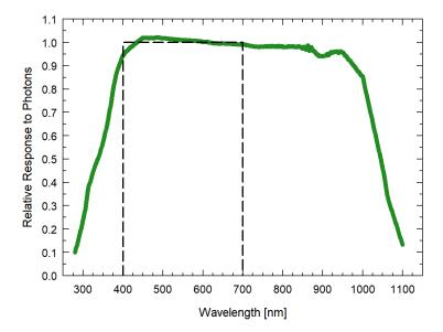
Mean spectral response measurements of six replicate Apogee SQ-600 series Quantum Light Pollution Sensors. Spectral response measurements were made at 10 nm increments across a wavelength range of 300 to 1100 nm in a monochromator with an attached electric light source. Measured spectral data from each quantum light pollution sensor were normalized by the measured spectral response of the monochromator/electric light combination, which was measured with a spectroradiometer
