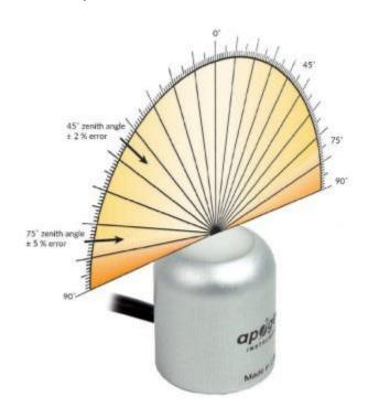
Directional, or cosine, response is defined as the measurement error at a specific angle of radiation incidence. Error for Apogee SQ-600 series Quantum Light Pollution Sensor is approximately  $\pm$  2 % and  $\pm$  5 % at solar zenith angles of 45° and 75°, respectively.
