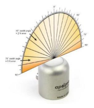
Directional, or cosine, response is defined as the measurement error at a specific angle of radiation incidence. Error for Apogee SQ-600 series Quantum Light Pollution Sensor is approximately  $\pm 2$  % and  $\pm 5$  % at solar zenith angles of 45° and 75°, respectively.
