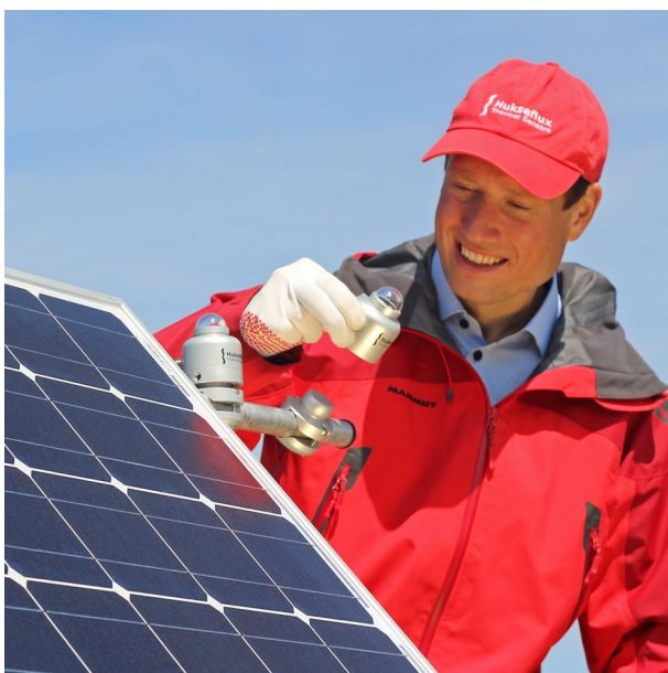
Figure 2 SR05's, one in PoA, replacing PV reference cells
