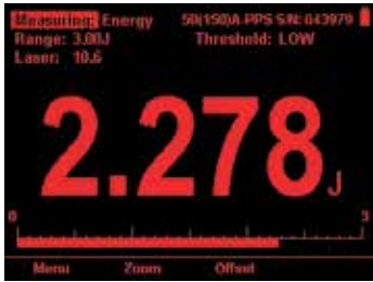
Bargraph display of energy. Colors set for work with protective glasses.
