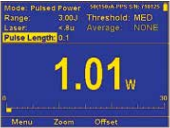
Power measurement of laser pulse. For use with high-power pulsed lasers.
