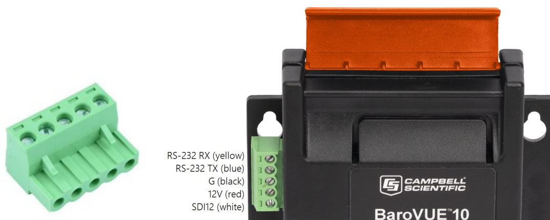
Figure 7-1. 5-pin screw terminal plug connector and connections
