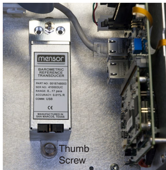
Figure 8.5.3.2 - Internal Barometric Reference
