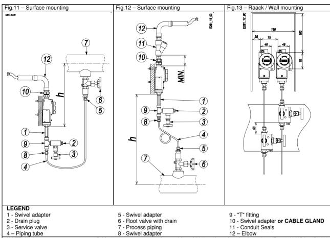
NOTE: With gas or vapour process fluid, the instrument must be positioned higher than the pipe inlet (see Fig. 12). With a liquid process fluid, the instrument can be positioned higher or lower, indifferently (see Fig. 11 and 12). In this case, during set point calibration the negative or positive head must be taken into account (distance h in Fig.11 and 12).
