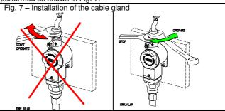
Tightening the cover as the wiring of the instrument is finish checking the position of the cover O-ring.
