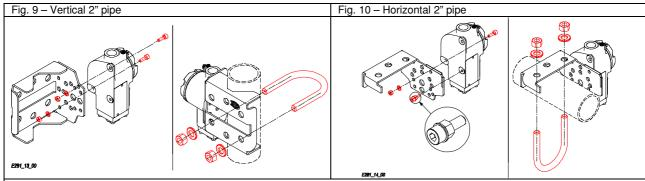
**Note:** To install the instrument on the 2" pipe use the mounting brackets accessories supplied with the instrument. To mount the instrument on the brackets use the M5 screws supplied as per Fig. 9 or 10.
