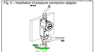
Carry out the connection using a flexible tube in such a way that the tube itself does not apply a force the instrument process connection due to variations in temperature.
