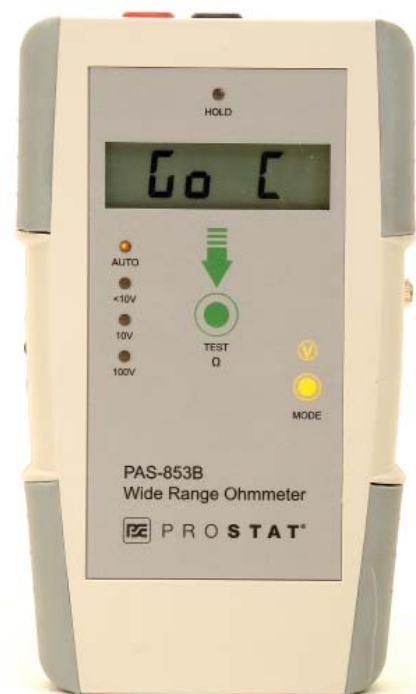
Figure 3: PAS-853B in Continuous Operation Mode
