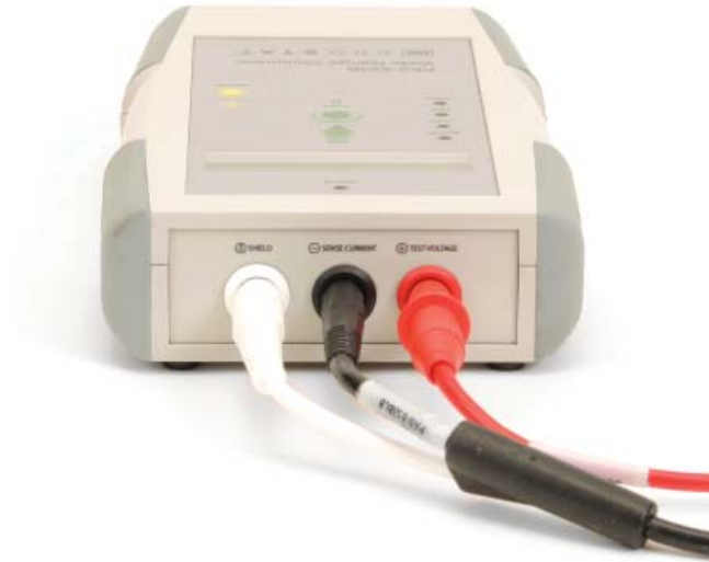
Figure 9: The shield is connected to the meter via the White banana plug and receptacle
