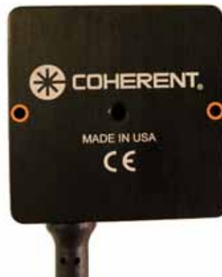
Figure 2-10. Sensor Housing Mount Drill Holes
