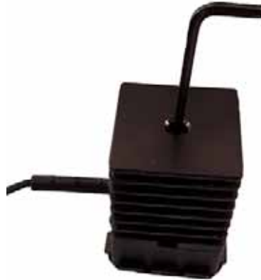
Figure 2-9. Attach Heat Sink
