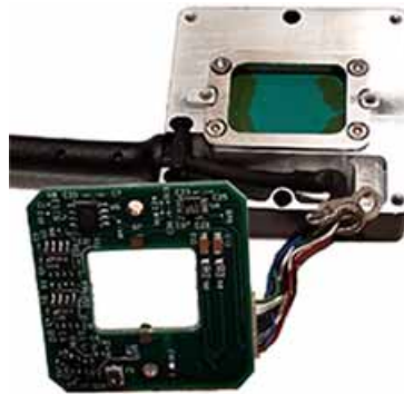
Figure 3-8. Remove the Circuit Board from the Sensor
