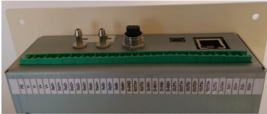
Figure 19: Connection socket for an external HC2 probe
