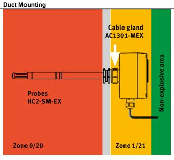
Use the accessory AC1301-MEX (mounting gland for 15 mm ATEX probes) for zone separation.
