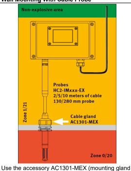
for 15 mm ATEX probes) for zone separation.
