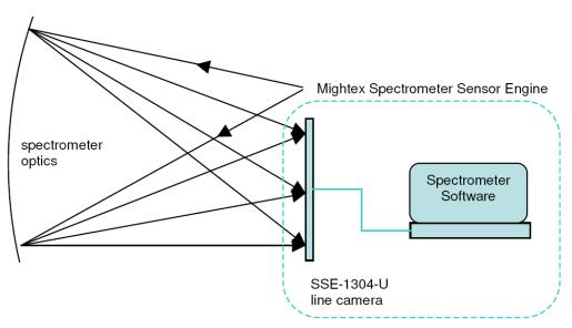
To build a complete spectrometer user will set up his own optics (spectrograph) and place the linecamera at the focal plane of the spectrograph. The spectrometer software provides a powerful set of spectrometer functions such as wavelength calibration, dark/bright references, spectrum display, and file management. Mightex SSE releases users from the burden of programming spectrometer functions so that they are able to build their spectrometers much more efficiently and cost- effectively.
